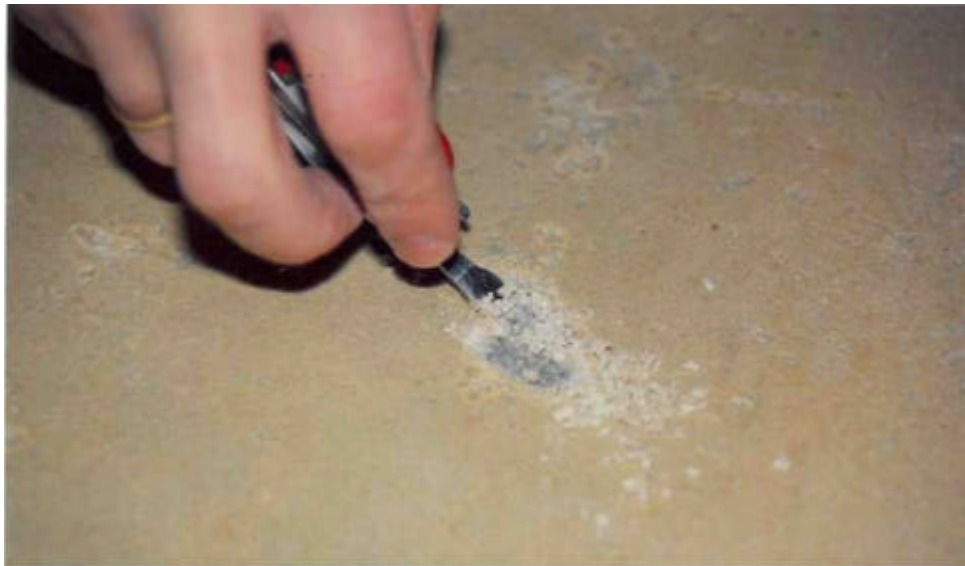
Figure 3: Softened material from a damaged area that can be easily removed manually.
